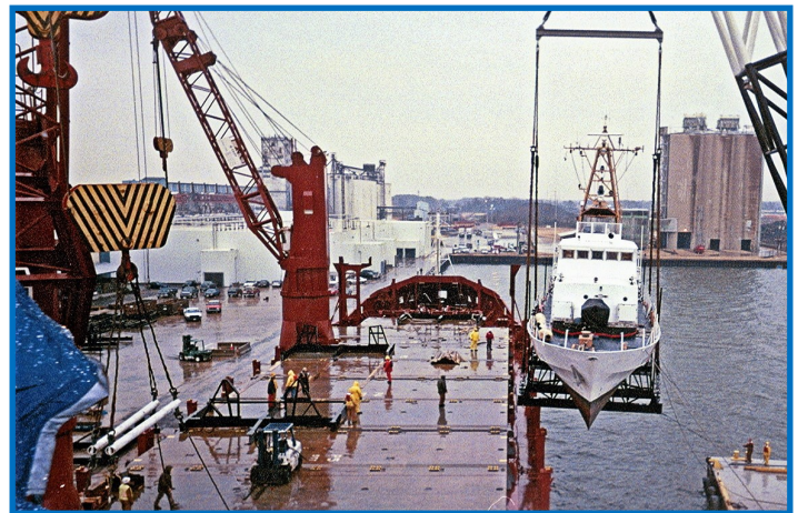
Heavy-lift crane loading 110-foot patrol boat Adak onto Motor Vessel Industrial Challenger in Portsmouth, VA. (U.S. Coast Guard)
